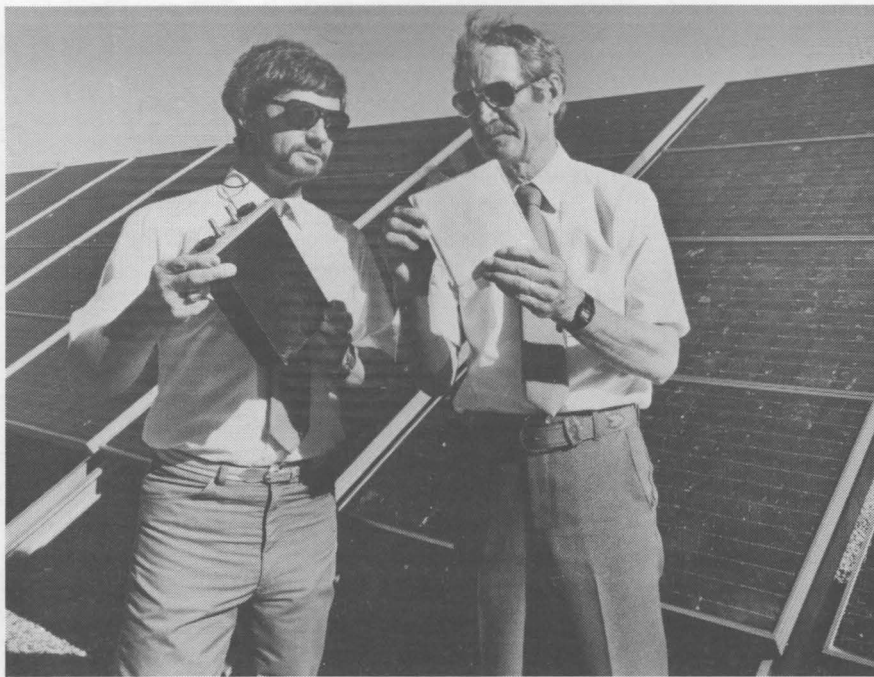
DON BUSH (2525, right) displays one of the nine "packets" that make up the nickel/hydrogen battery cell held by Ward Bower (6223). Ten such cells compose the 7-kWh battery currently under test in a cooperative experiment by Storage Batteries Div. 2525 and Photovoltaics Systems Research Div. 6223. The battery, located in Bldg. 833, is linked to the photovoltaic array shown behind Don and Ward and to a small refrigerator and four 30-watt fluorescent lights to simulate a remote-site photovoltaic system.
